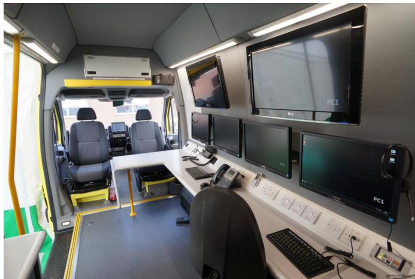
Figure 5: Ground Vehicle based Control Station (previous supplier contract)
